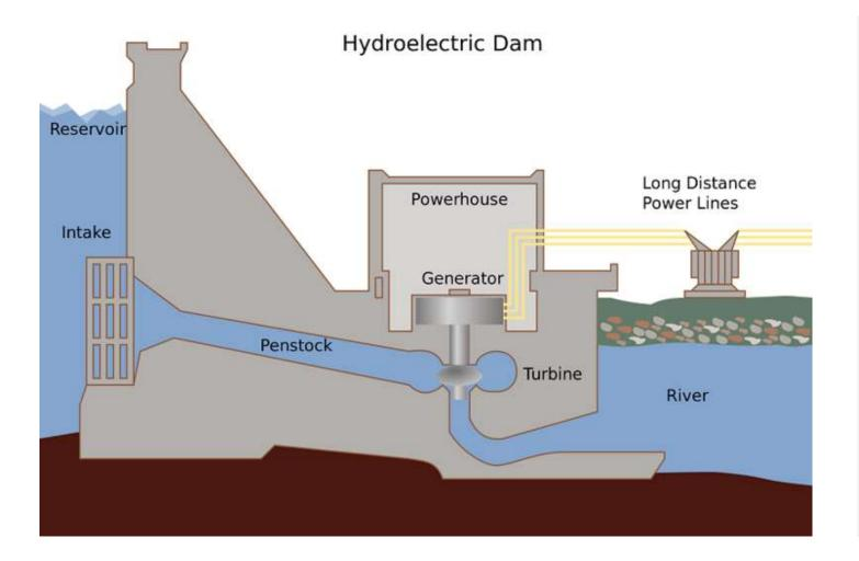
The hydroelectric power plant consists of a tank with water, where there is also a cap that admits the water into the supply channel, which leads to the turbine that turns it. The turbine is connected to the rotor of the generator and it creates an electric current which is discharged into the network. The water from the turbine flows further into the river further into the world.
